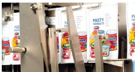
Cutting device, gripper and servomotor film pulling system are automatically adjusted from the machine touch screen with only one touch, thus ensuring a quicker format change.
