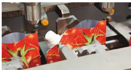
Dosing units for liquids available with different nozzles for any kind of product. Hygienic design and easy to dismantle filling system, with clamps. Bossar HFFS machines are suitable to work with different kinds of dosing systems: volumetric dosing units, multihead weighers, piston pumps fillers, etc.
