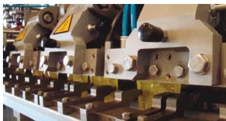
Top sealing and cooling groups with 180° folding hinge for easy cleaning. Sealing jaws adjustments are not required during the change of the sealing bars. Removable walking beam allows a fast format change over.
