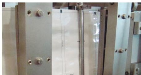
Vertical sealing group equipped with motorized size adjustment through touch screen. Sealing jaws temperature individually controlled.
